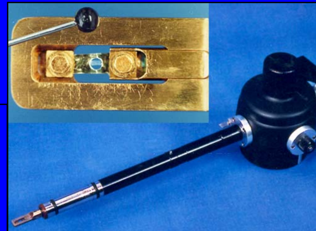
Transmission Electron Microscope Straining Holder Model 671 (Gatan) Temperature: -180 °C ... 120 °C Thickness: 100 nm ... 0.5 \mu m
